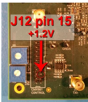
Figure 1: Location of +1.2V RF PA Enable Signal
