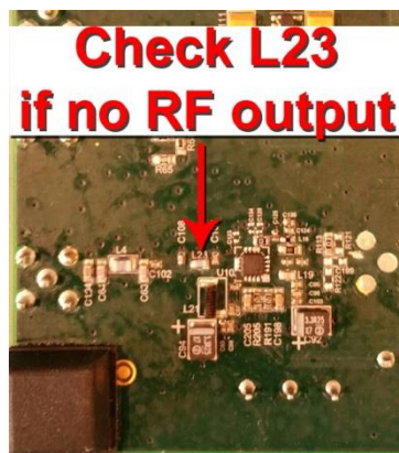
Figure 11: Where to check if no RF output is present
